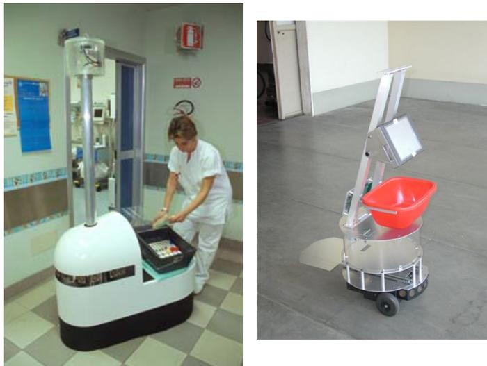
Figure 3 The Staffetta robot used in the HCI scenario (left), and the modified ActiveMedia Pioneer robot for the RDE (right).
